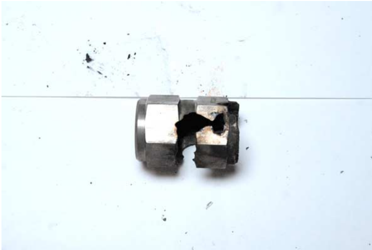
FIG. 6— Post-test condition of a stainless steel inline filter (View 1).
