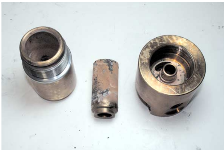
FIG. 9— Post-test condition of a brass tee type filter.
