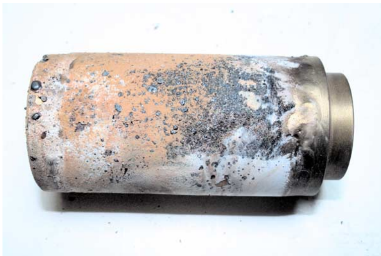
FIG. 10— Post-test condition of a brass tee type filter element (View 1).
