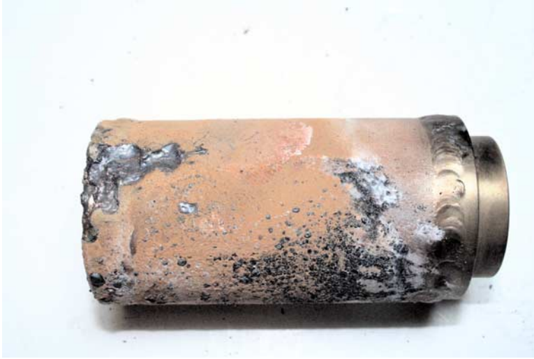
FIG. 11— Post-test condition of a brass tee type filter element (View 2).
