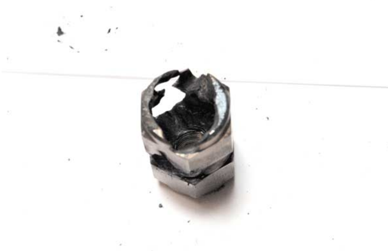
FIG. 7— Post-test condition of a stainless steel inline filter (View 2).
