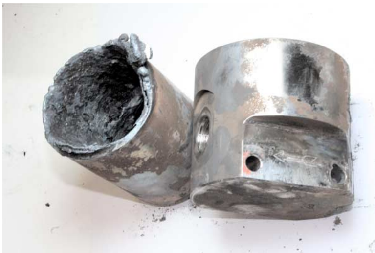
FIG. 4—Post-test condition of the stainless steel tee type filter (View 2).
