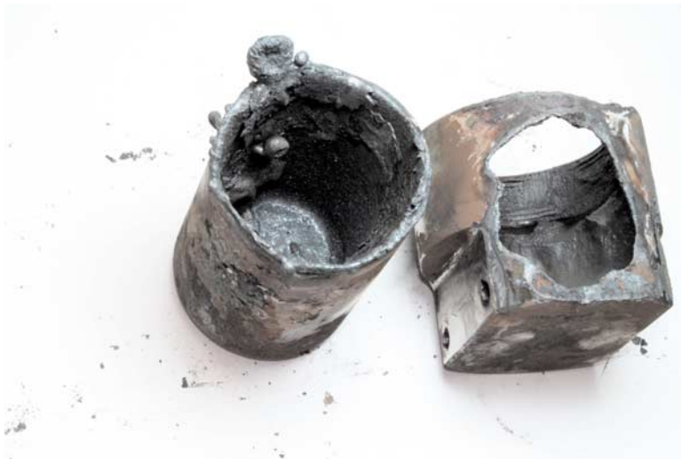
FIG. 3—Post-test condition of the stainless steel tee type filter (View 1).
