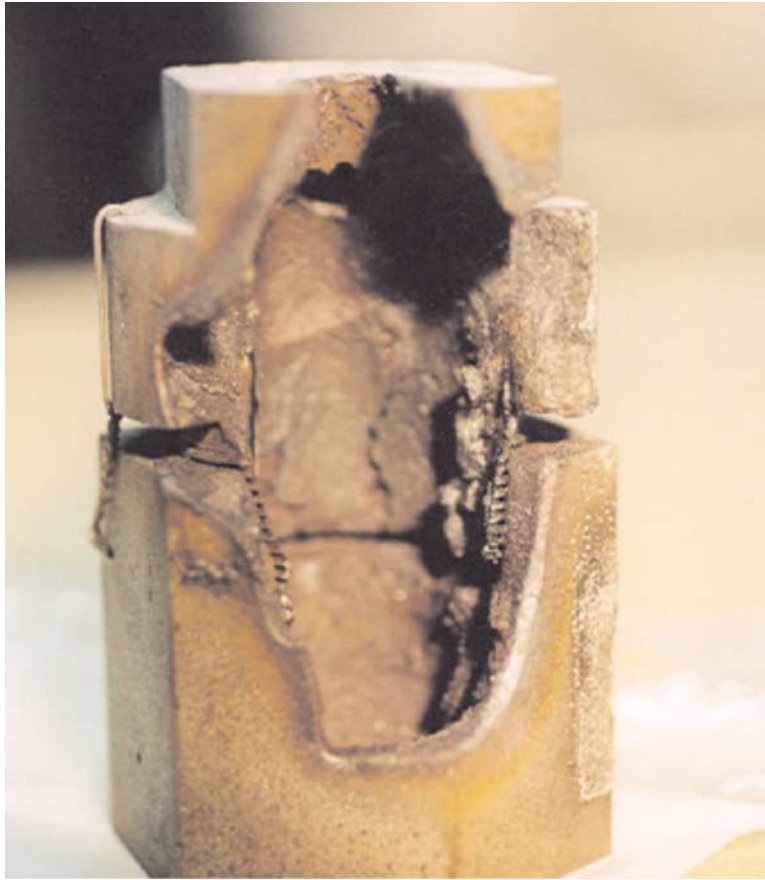
FIG. 1—Condition of a breathing gas booster filter after an ignition in the field.
