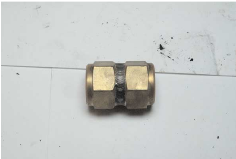
FIG. 13— Post-test condition of a brass inline filter (View 1).
