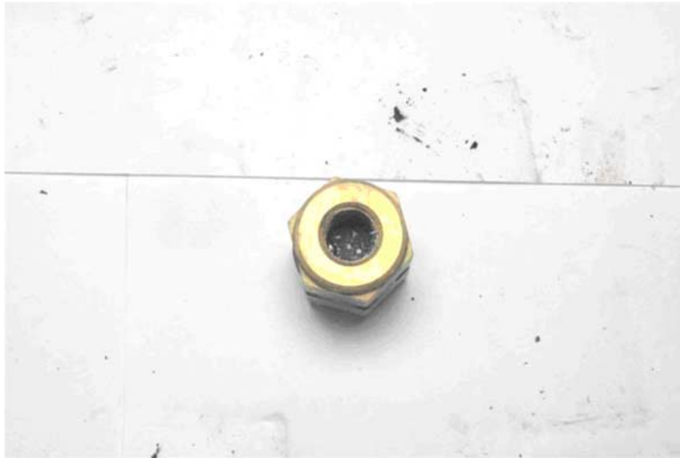
FIG. 14—Post-test condition of a brass inline filter (View 2).
