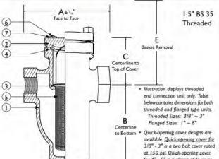
for 4" - 8" is a clamp style cover. rated at 200 psi Four balt cover is shown and is standard.
