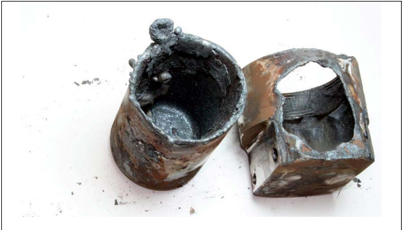
Photo 7: Post-test view of test article TA-ST-1 (Stainless Steel Tee Filter).
