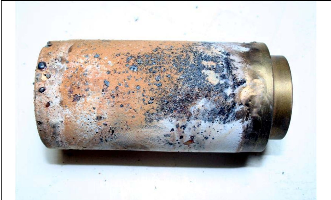
Photo 16: Post-test close-up view of test article TA-BT-2 filter element (Typical).
