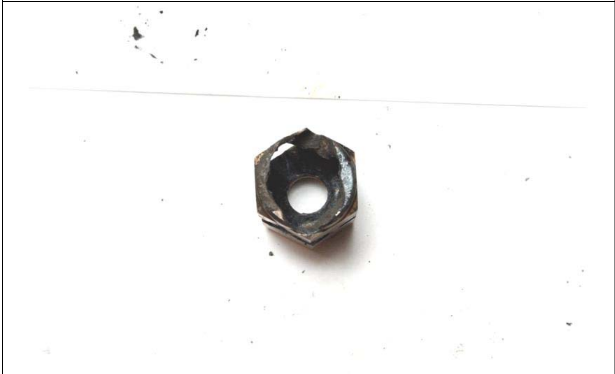
Photo 14: Post-test view of test article TA-SI-1 (SS Inline Filter).
