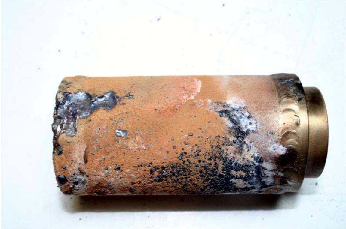
Photo 17: Post-test close-up view of test article TA-BT-2 filter element (Typical).
