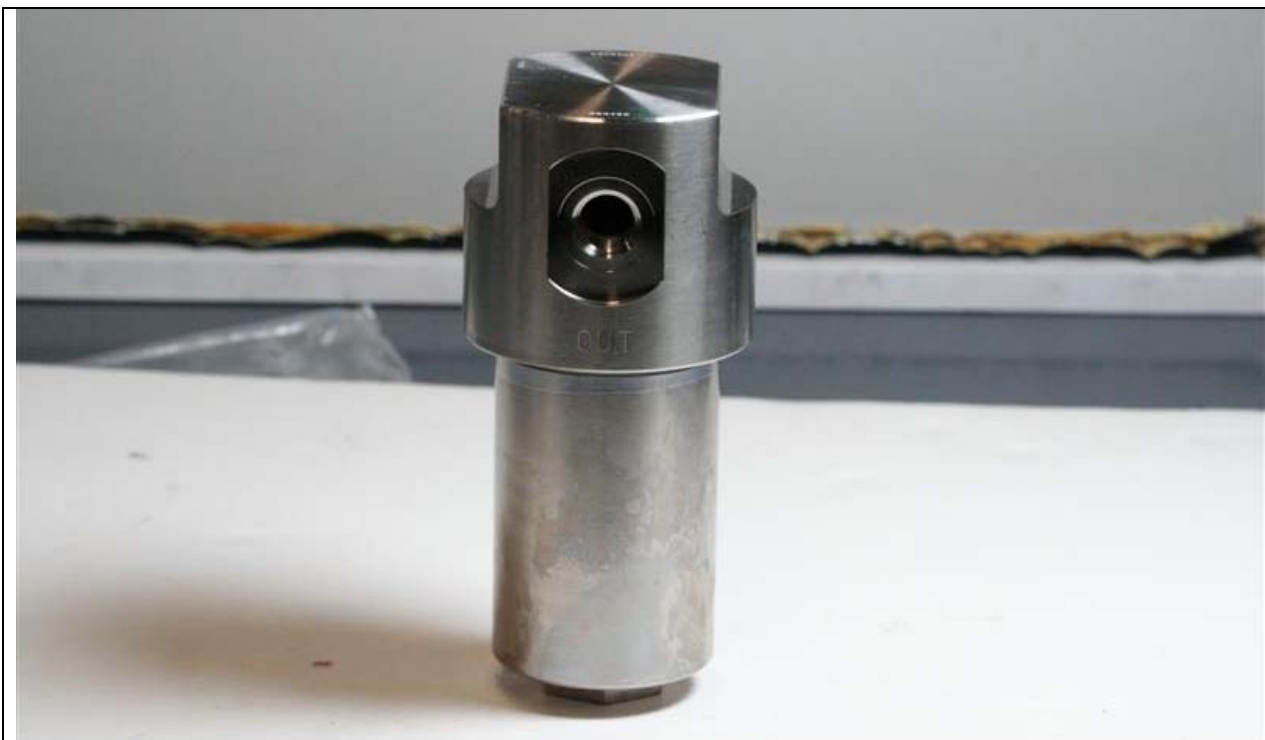
Photo 1: Typical Stainless Steel Tee Type Filter in its “as received” condition.
