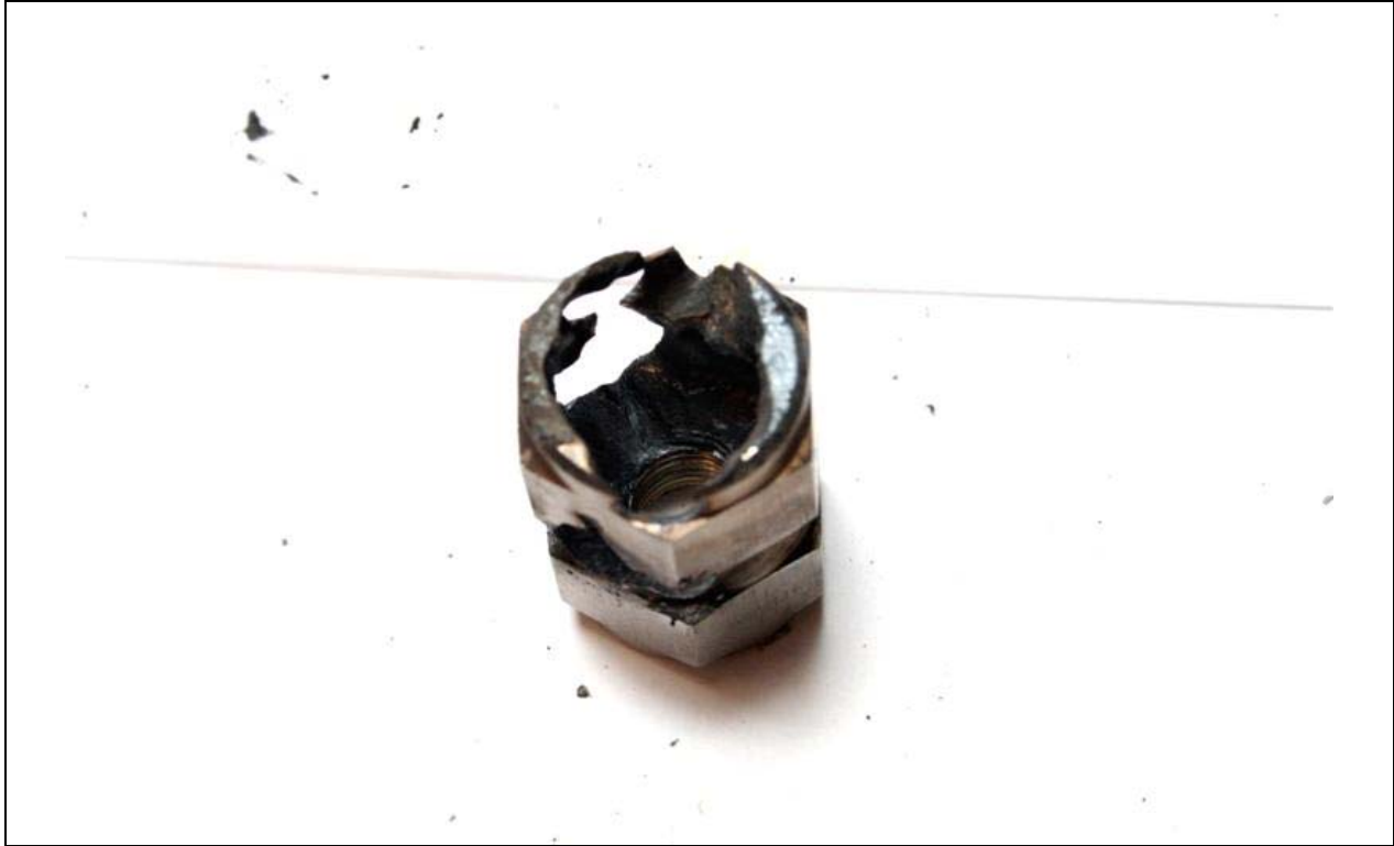
Photo 13: Post-test view of test article TA-SI-1 (SS Inline Filter).
