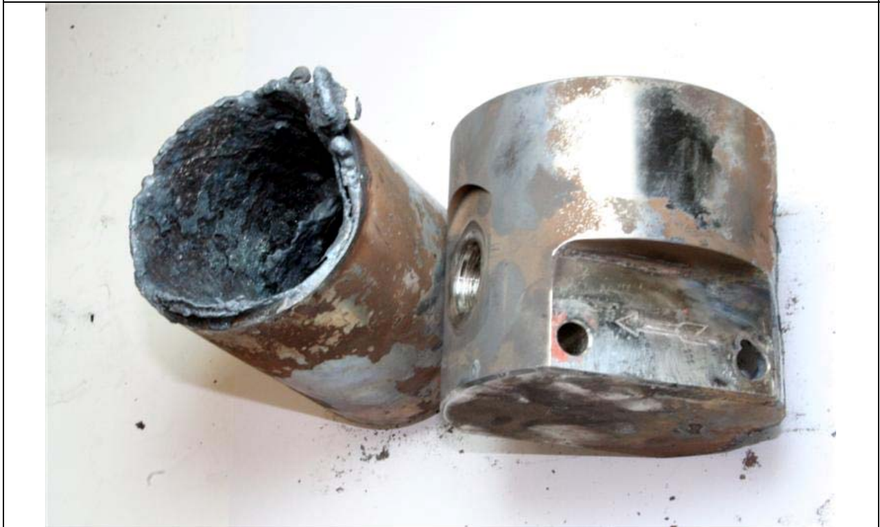
Photo 8: Post-test view of test article TA-ST-1 (Stainless Steel Tee Filter).
