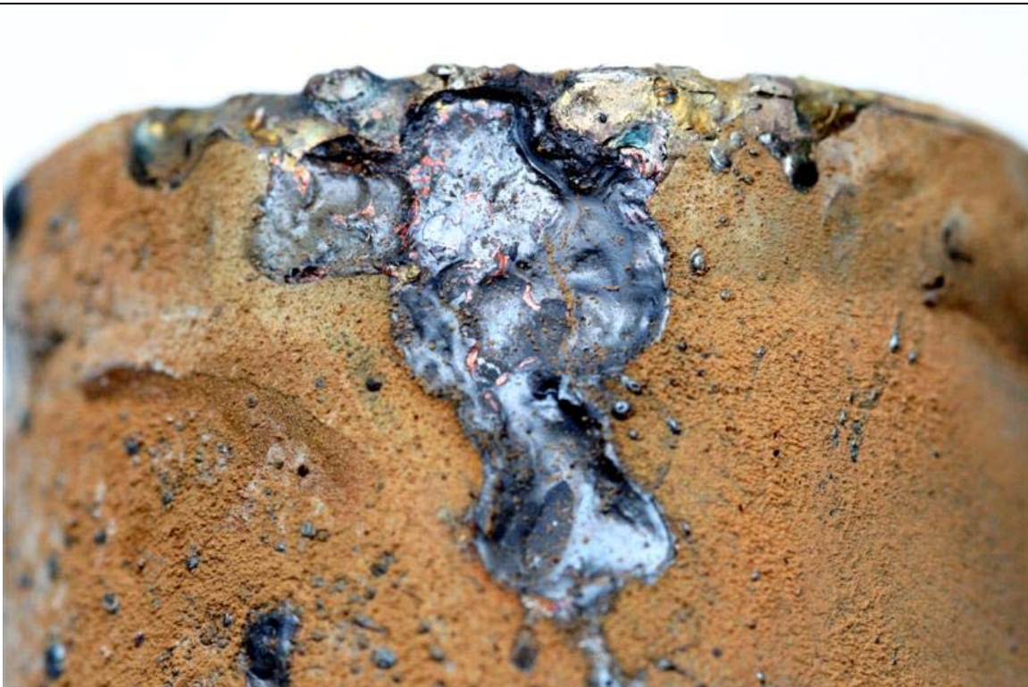
Photo 18: Post-test close-up view of test article TA-BT-2 filter element.
