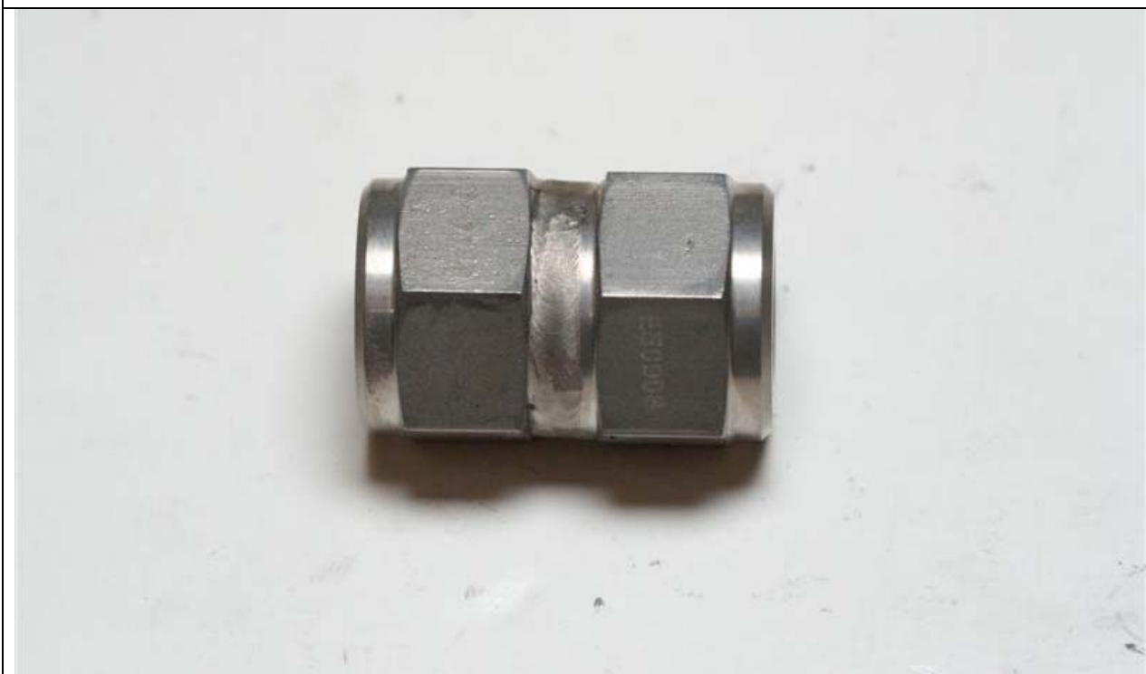
Photo 2: Typical Stainless Steel Inline Filter in its “as received” condition.
