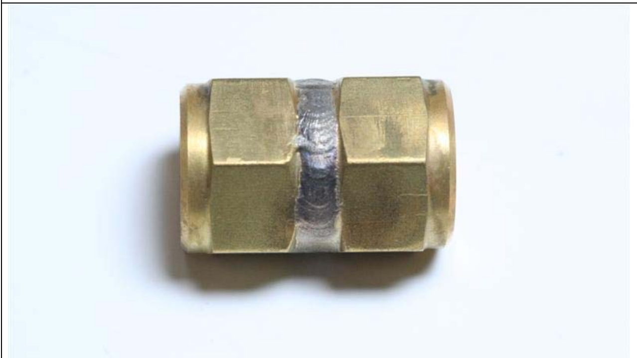
Photo 4: Typical Brass Inline Filter in its “as received” condition.
