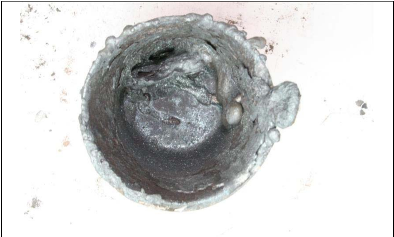
Photo 9: Post-test view of test article TA-ST-1 (Stainless Steel Tee Filter Housing).
